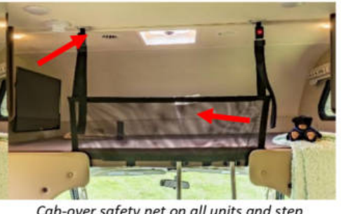
Cab-over safety net on all units and step ladder to get into cab-over area
